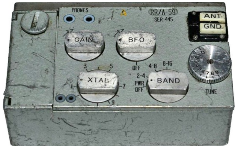
The here shown A-model receiver RR/A-59 differed not much from the later RR/C-59 model pictured on the previous page. (above) Pins on the top side connected the receiver with the BS-59 Interface unit. (below)
