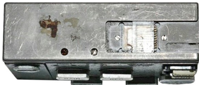
The here shown A-model receiver RR/A-59 differed not much from the later RR/C-59 model pictured on the previous page. (above) Pins on the top side connected the receiver with the BS-59 Interface unit. (below)
