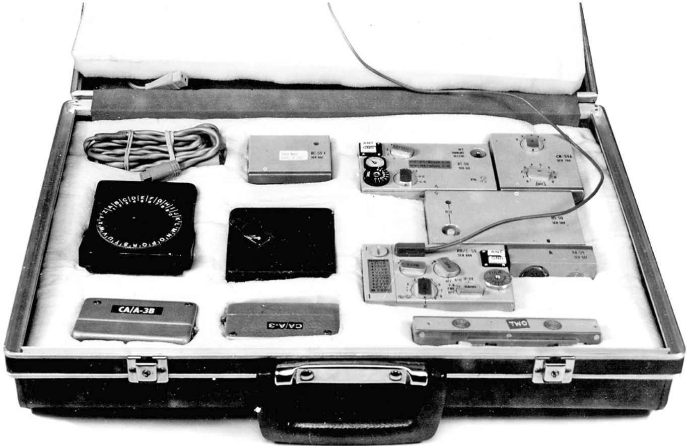
Complete fully transistored agents station RS-59 packed in a suitcase. This particular suitcase was captured in the GDR in possession of an American agent.
